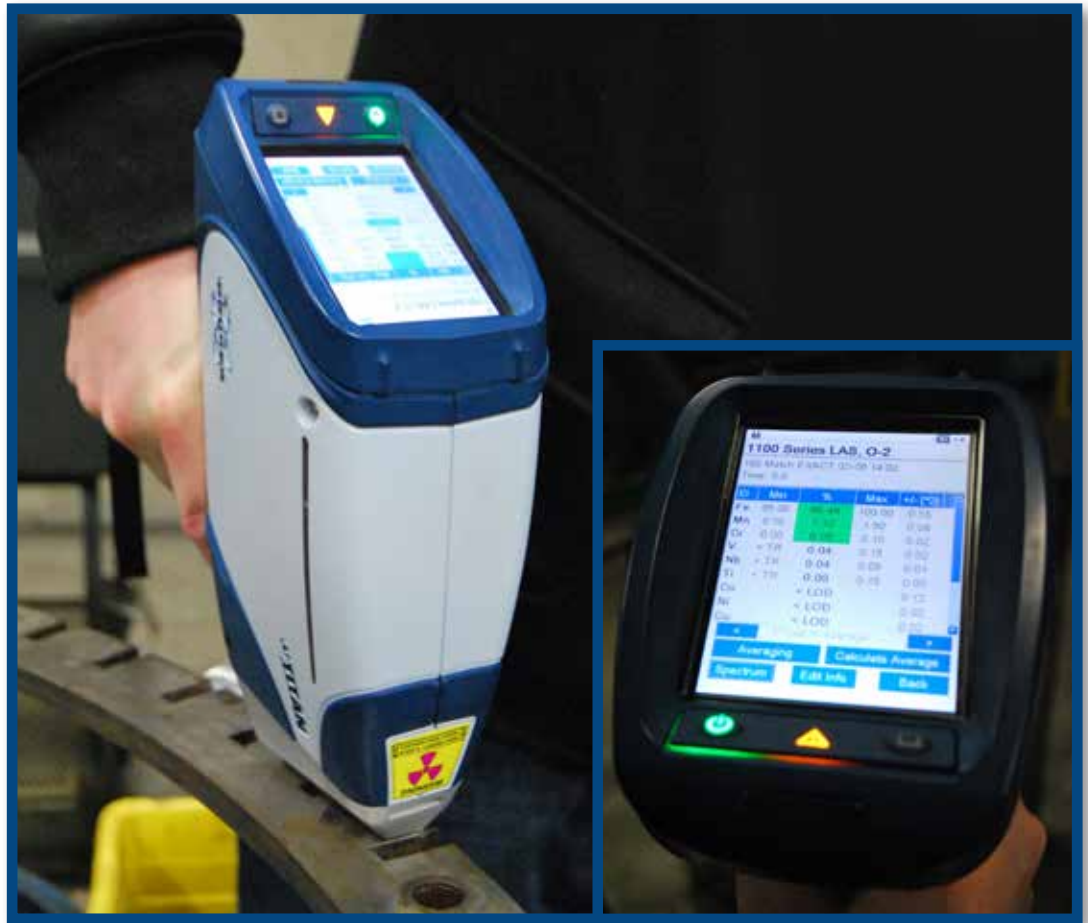
Metal being tested for composition by Engineering Services.
