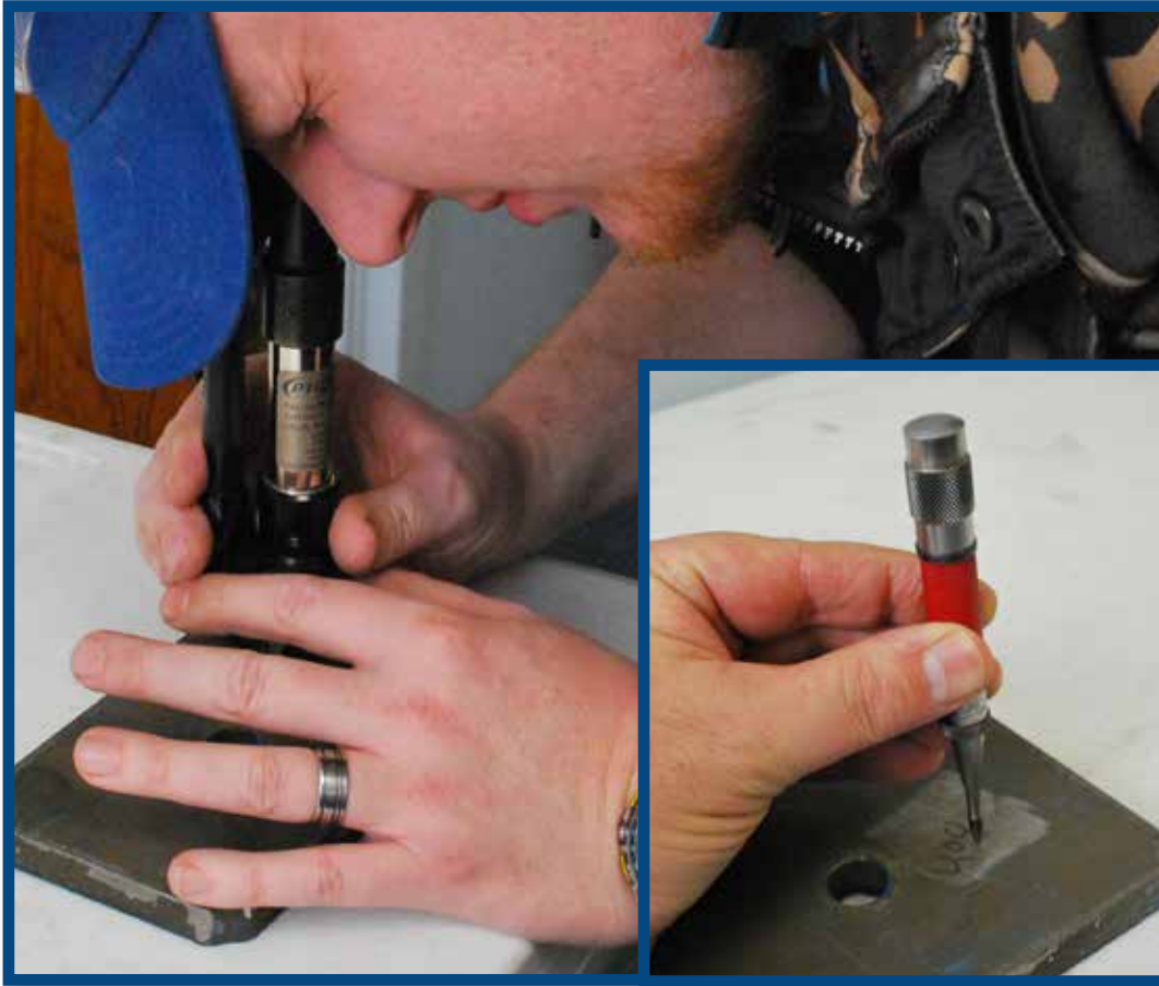
Metal being tested for hardness by Engineering Services.
