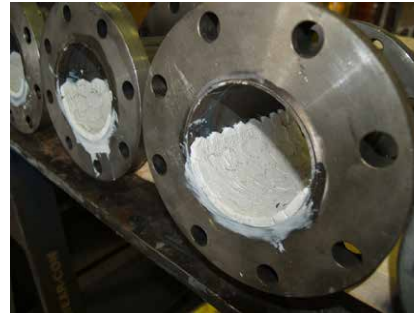
Flop Gate lined with WC90™ HexTile Ceramic
