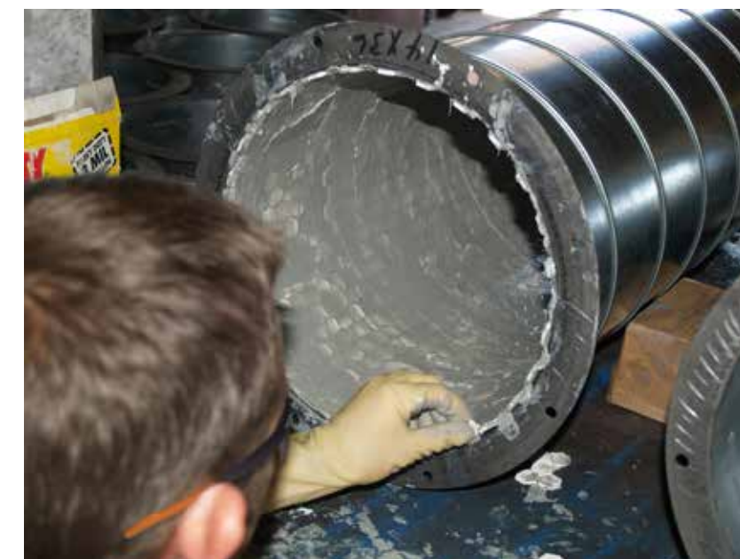
Transition Spool lined with WC90™ HexTile & WC90™ Plain Ceramic
