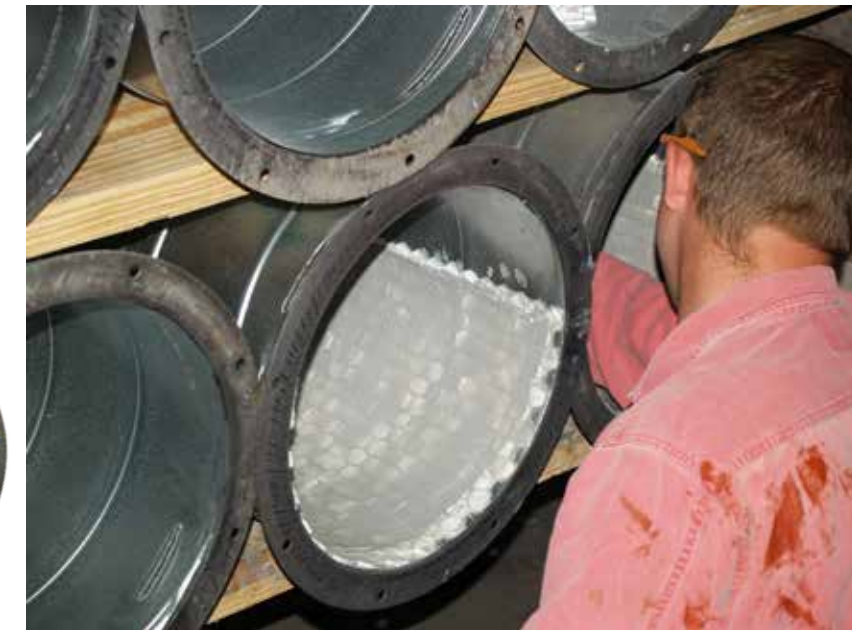
Flop Gate lined with WC90™ HexTile Ceramic
