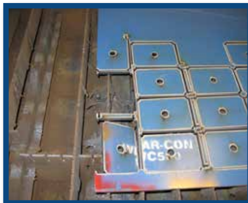
WearPads cut out of WC500™ Plate.
