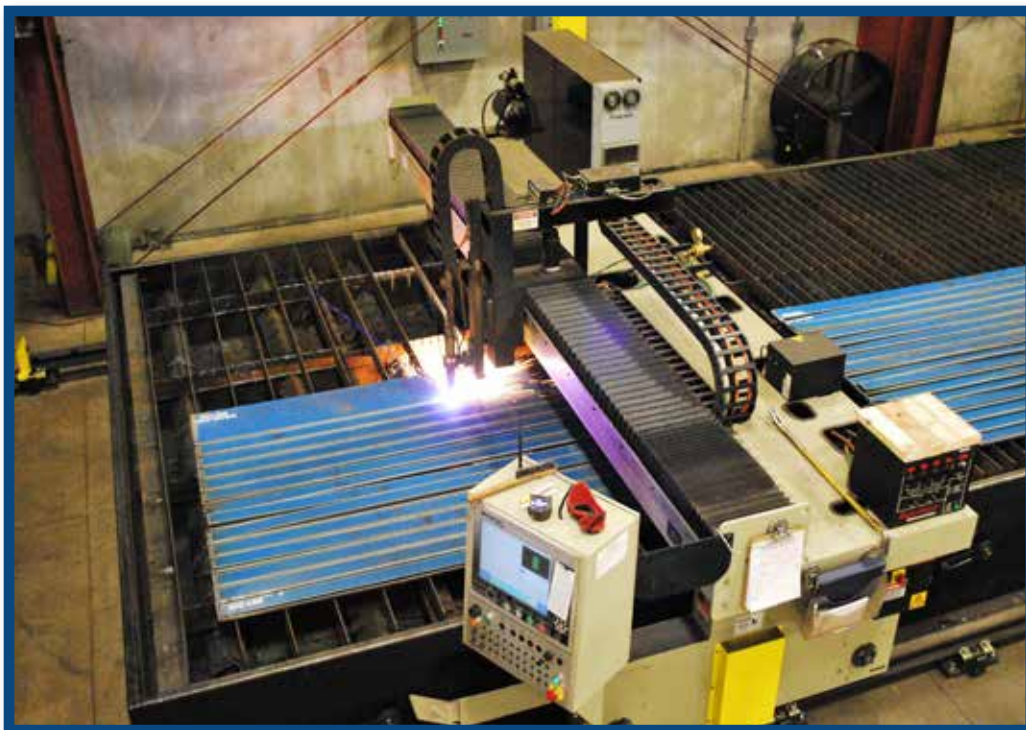
Wear-Con's Plasma Cutter cutting a series of WearStrips out of WC400™ Plate.
