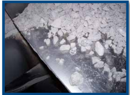
INERTIA™ Tactical Wear Plate installed in feeder.
