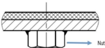
**COUNTERBORE OF WEAR PLATES:** cut through hole with line cutting, embed countersunk ring and weld to nut base with E7018 or E70-s rod
