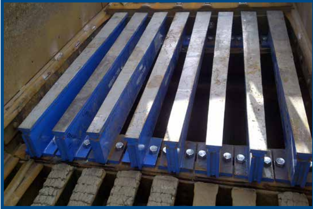
Grizzly/Grouser Bars installed.
