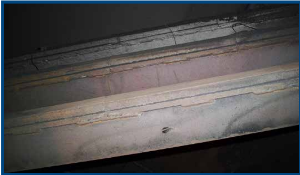
Installed Grizzly/Grouser Bars capped with WC810™ .
