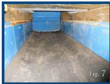
h a r d - e n e d material that has slow wear attributes and actually polishes the skirtboard over time to provide a much smoother edge near the belt surface. The added benefit to this chemistry also provides a corrosion resistant covering against the wet coal during the spring and fall months. Increasing numbers of **SHC800™** Inner SkirtBoard Panels are being installed with great success.
