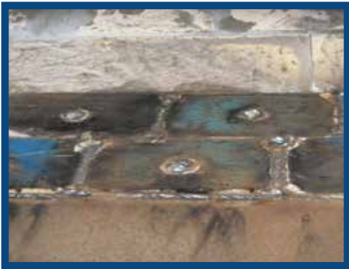
WearPads™ used to patch worn area.
