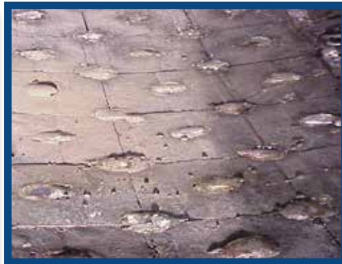
Prop Pump lined with WearPads™
