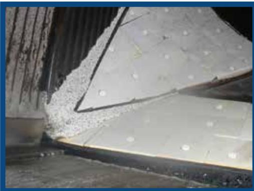
After years of service, **TB90™** transitioning between **WC90™** Weldable Ceramic.
