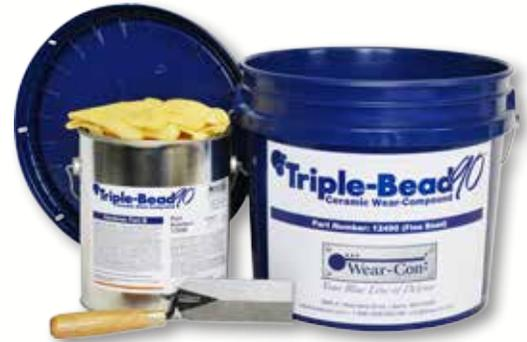
Wear-Con **Triple-Bead90™** is easy to mix and install. Simply mix one part **TB90™** Resin - Part A with one part **TB90™** Hardener - Part B and trowel on. **Triple-Bead90™** is workable for up to forty five minutes.
