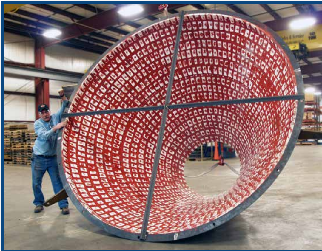
Classifier Cone Lined with WC90™ Weldable Ceramic Wear Tiles.
