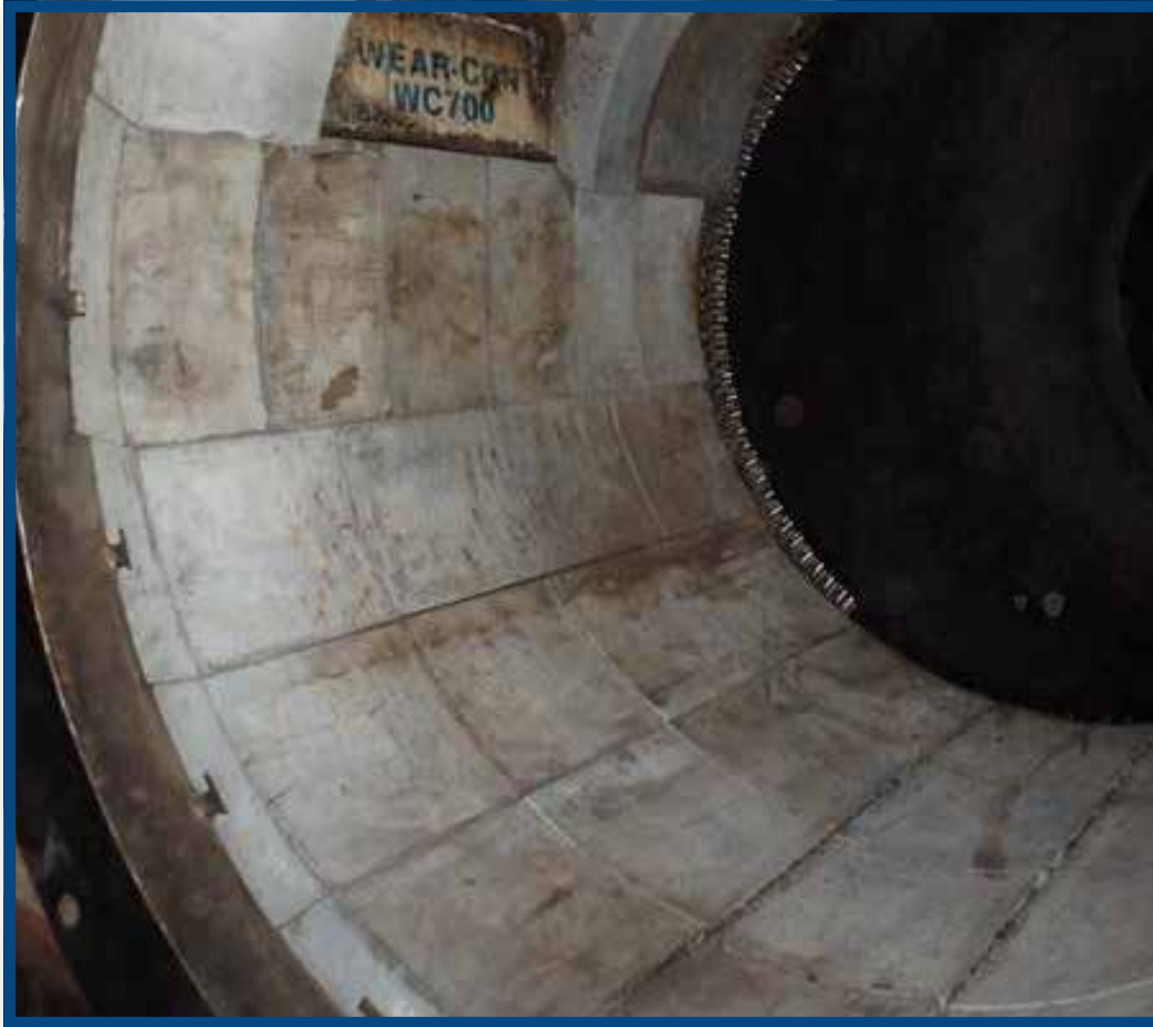
Burner nozzle lined with WC88R™ .
