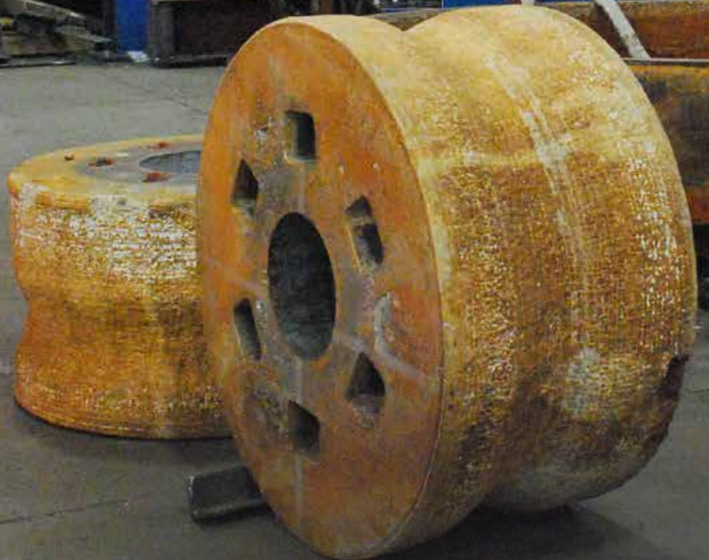
Worn Mill Rolls staged to be rebuilt in front of rebuild area.
